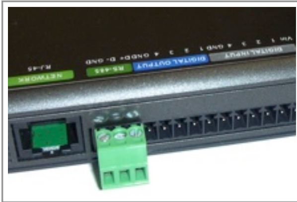
Figure 1 Outlook of the BRIDGE
