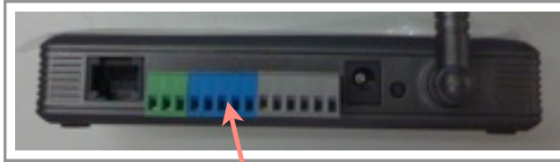
Digital output port must be disconnected to any wire
