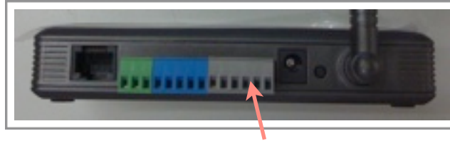
Digital Input port must be disconnected to any wire
