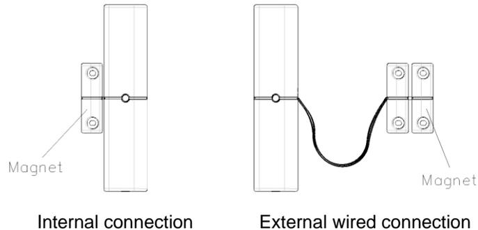
Choose either the internal or external wired connection, both of which types cannot be in existence at the same time.
